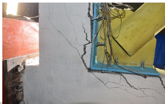
Fig. 2: Diagonal crack at beam-column joint
