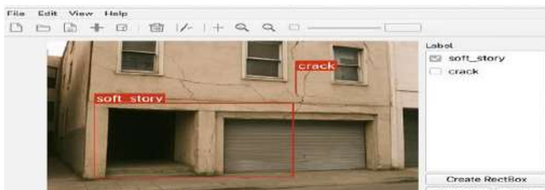
Figure 1: Manual annotation of training data using bounding boxes to label seismic vulnerabilities
