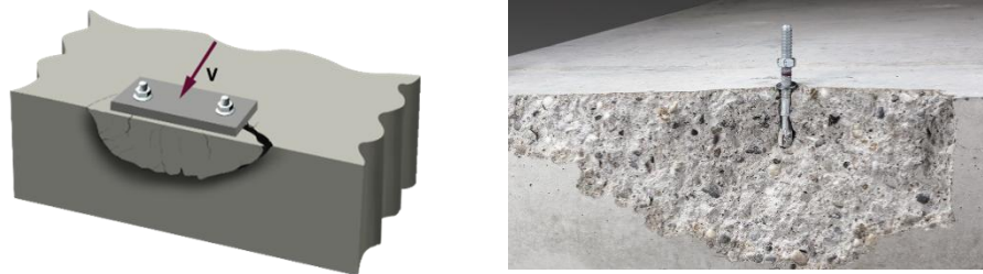
Fig. 3.20: Concrete Edge failure under shear loading
