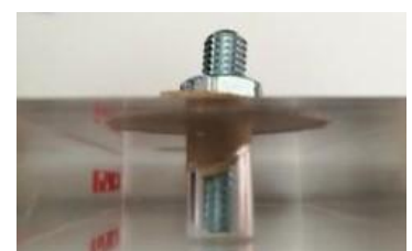
c) Unsuitable filling method used
