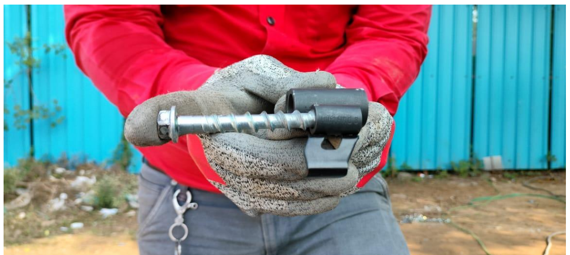
b) Hilti anchor with re-usable gauge
