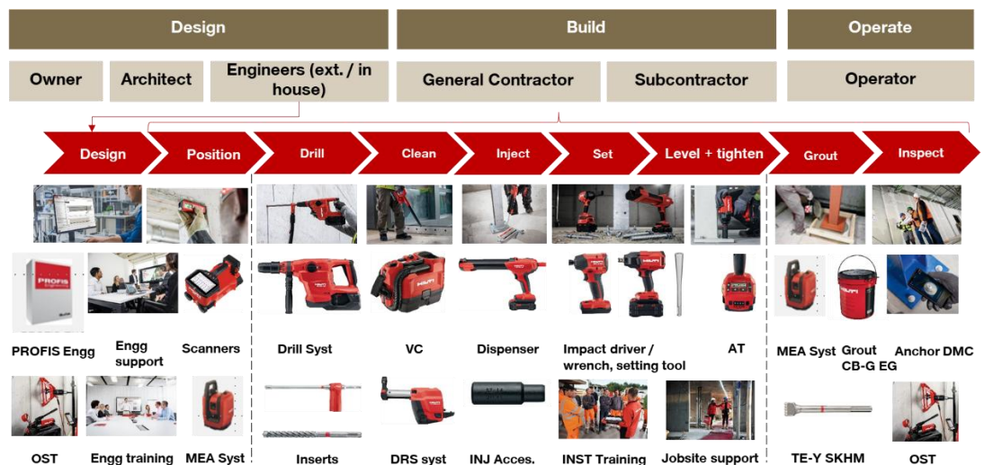
Fig. 8.2: Flowchart for installation of post-installed anchors
