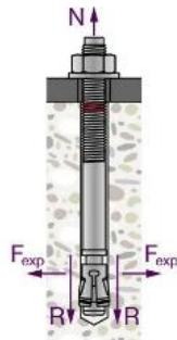
Fig. 3.4: Torque-controlled expansion anchor
