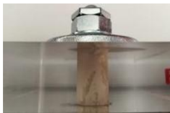
b) Hilti filling set in use Fig. 5.2: Hilti Filling set
