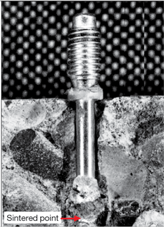
Fig. 4.5 Example of Sintering [24]
