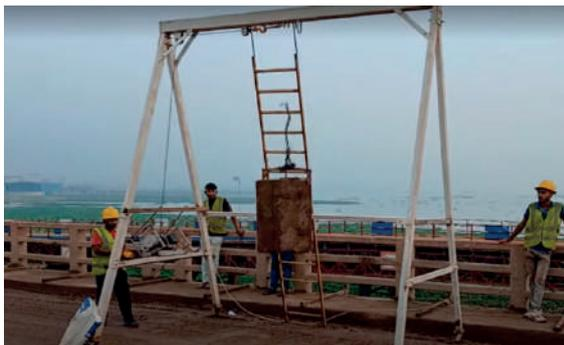
Fig. 17: Heavy object being dropped for the impact load test
