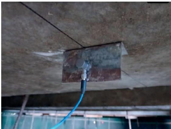
Fig. 14: ICP Accelerometers attached to the girders
